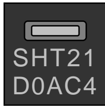
Figure 19 Laser marking on SHT21. For details see text.
