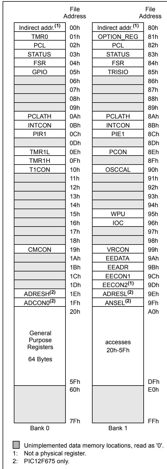
FIGURE 2-2: DATA MEMORY MAP OF THE PIC12F629/675
