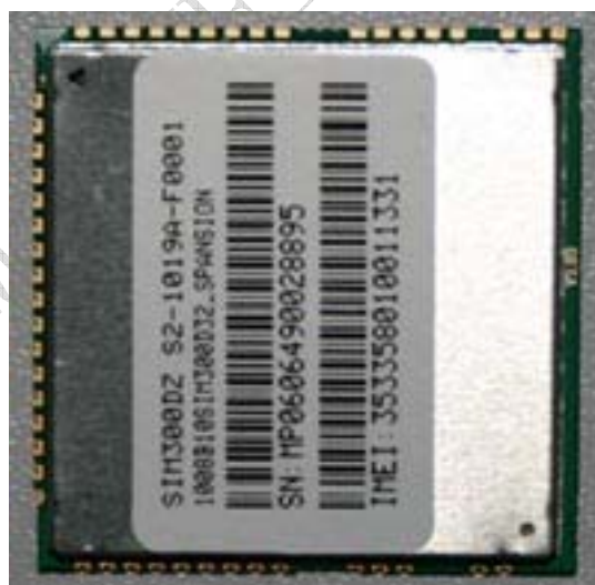
Figure 31: Bottom view of SIM300DZ
