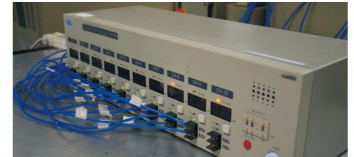
Electric Current Break Test Equipment
