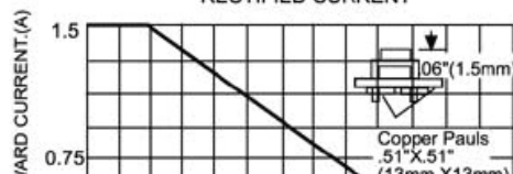
FIG.1 - MAXIMUM DERATING CURVE FOR OUTPUT RECTIFIED CURRENT
